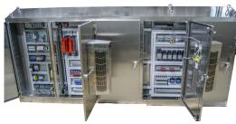
This panel was built for process and motor control of a bottling line in the food industry. ECT provided designed assistance and fabricated the panel.
