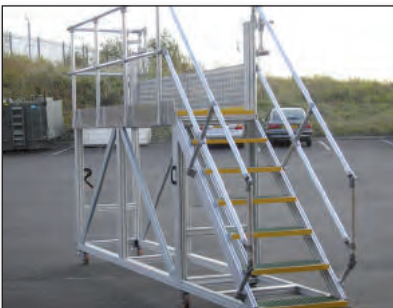
Flask inspection platform
